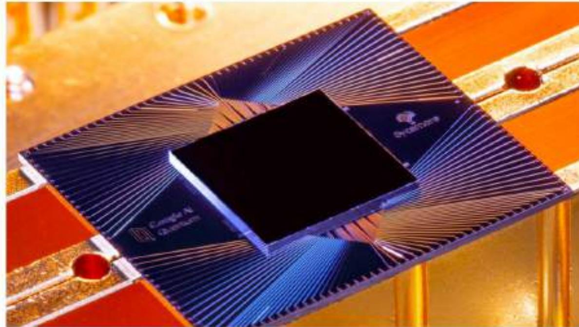
Google researchers report that their quantum computer, Sycamore, has performed a calculation that can't be achieved with any classical computer. The quantum chip (shown) must be cooled to near absolute zero to function.
